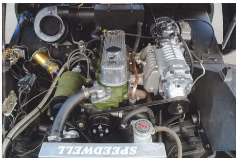
The supercharger increased the engine's output by an estimated 40 percent, from 65 hp to 90 hp.
