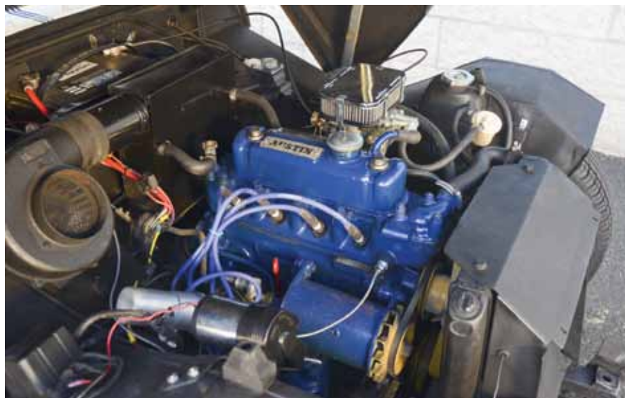
A Weber carburetor, a header and a performance cam give this 1,275cc four an estimated 75hp. A dual-pipe muffler lends it an aggressive rasp.
