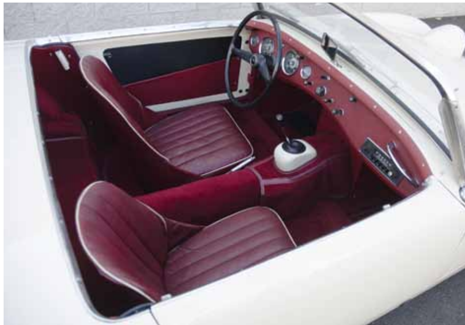
Craftsmanship and attention to detail hide the five-inch stretch added to this Bugeye's wheel-base. As with all Mk I Sprites, the only access to the trunk and spare tire is from the interior.
