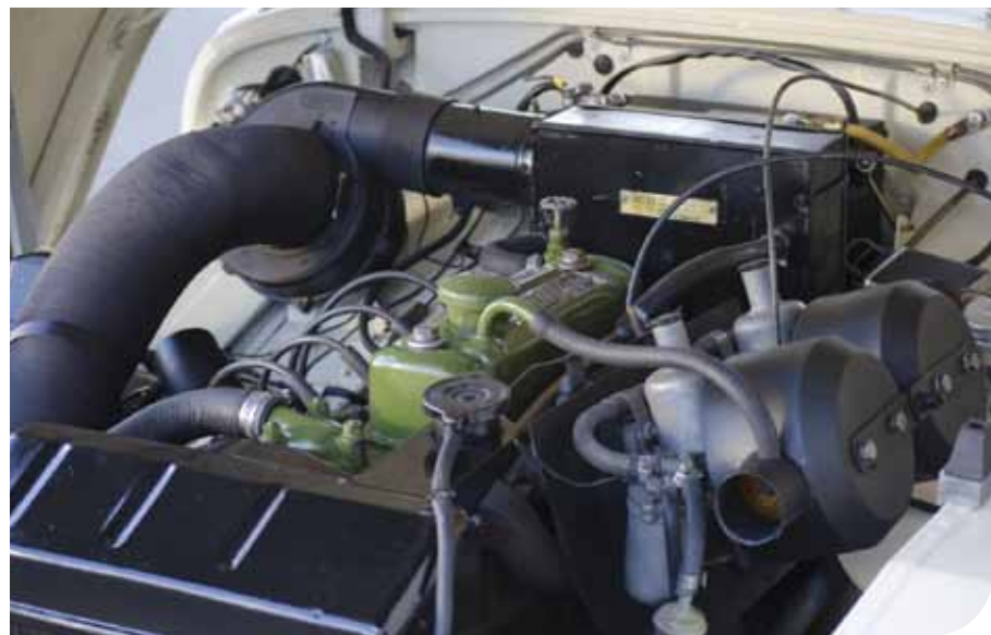
Like many Bugeyes, Dave Fite's car features a later 1,275cc inline-four. Visually similar to the 948, it makes nearly 50 percent more power.
